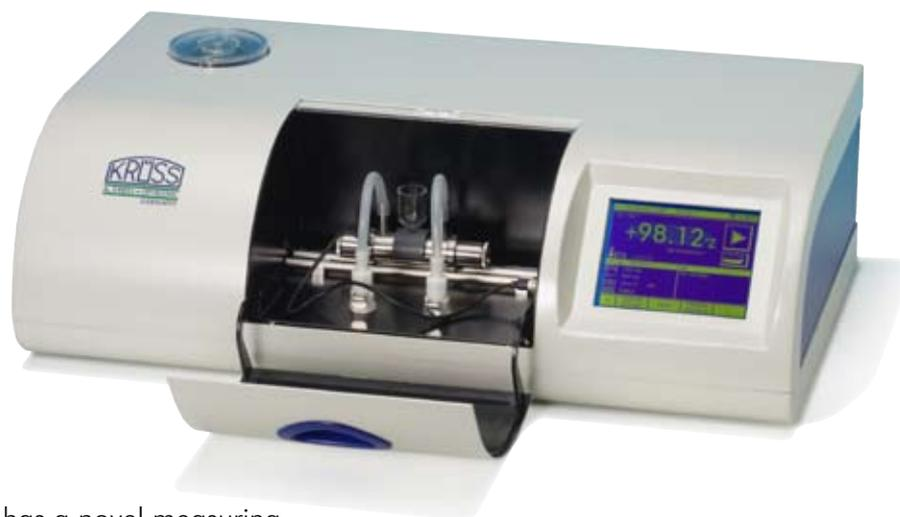
The new A. KRÜSS Optronic Sugar Polarimeter has a novel measuring principle for optically-active liquids. This latest development reduces the measuring time to one second, irrespective of the angle of a sample.
