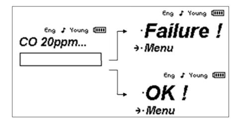
If the 20ppm calibration is successful, "OK!" will be displayed. Otherwise, "Failure" will be displayed. (If failure happens see the troubleshooting section)
