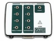
the system. An optional 8-channel DC input module, patient event button, and and optional pulse oximeter allow for an additional 13 channels of data. This flexibility allows for wide range of physiological parameters to be monitored and recorded.
