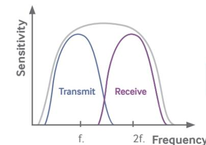
Transmit/Receive at conventional transducer
