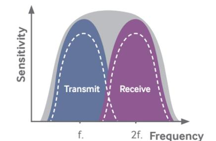
Transmit/Receive at S-Vue transducer
