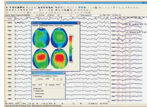
Neuron-Spectrum-LEP. Recording and analysis of multi-channel long-latency evoked potentials.
