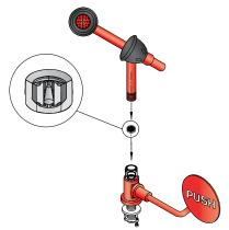
FLOWFIX is a feature that is built into most of BROEN's eye baths and hand/eye showers. Flowfix is a water regulating device, that controls the water flow at a preset rate regardless of water pressure.
