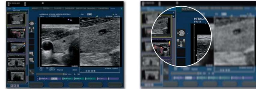
Detail of vertical toolbar: selection of probe/application, and simplified image transfer.
