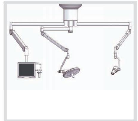
A SATELITE-based multimedia configuration: PowerLED 300, single flat screen and ORCHIDE HD camera.
