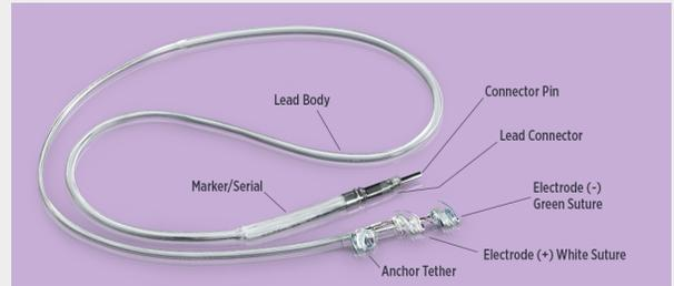
**The PerenniaFLEX (Model 304)** combines the flexible handling characteristics of early device models with 3.5-times greater durability over the previous LivaNova lead models. Bench testing of the PerenniaFLEX shows an average of 810,000 cycles to failure before electrode bifurcation fatigue, and an average of 76,000 cycles to failure before conductor coil fatigue.<sup>1</sup>
