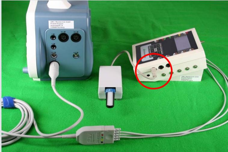
2.) Checking the SpO<sub>2</sub> function with the "SECULIFE pulse oximeter module". The nominal value of the FingerSim™ (here: 97 %) should approximately correspond to the value displayed at the DUT (here: 98 %).
