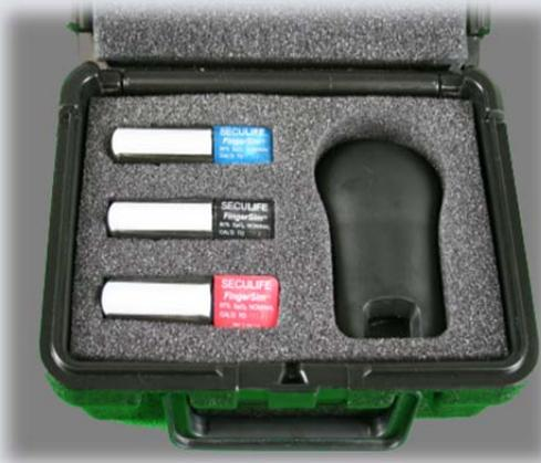
The FingerSim pulsoximeter-testing system enables the user to test pulsoximeters and sensors with three simulated light absorption conditions. These absorption conditions imitate typical oxygen saturations.
