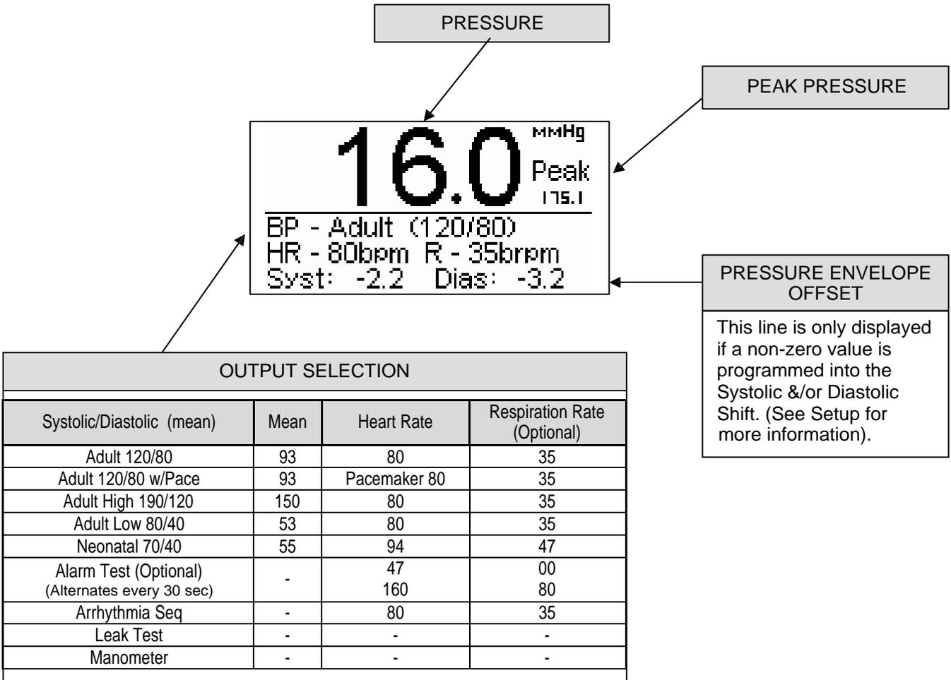
**OUTPUT WAVEFORM SCREEN** – This screen shows the pressure, peak pressure, output selection, and output waveform.
