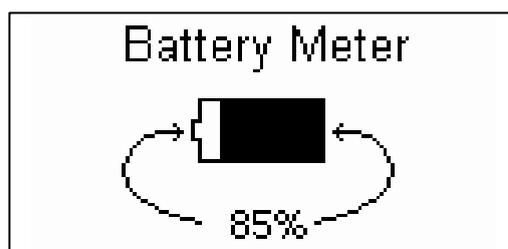
Batteries charge from provided AC power adapter. The charge time is about 4 hours from full discharge.
