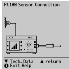
Temperature can be measured within a range of  $-200\text{ °C}$  to  $+850\text{ °C}$  with a Pt100 or Pt1000 sensor (default setting) connected to the PE (1) and N (2) jacks.
