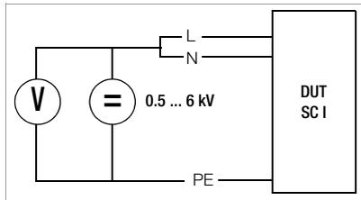
If safety class II is recognized, the test is conducted between the short-circuited conductors L-N of the test socket and the probe (connection 4-5).
