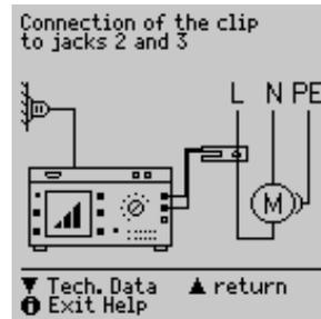
Alternating current can be measured in two measuring ranges (1 mA ... 10 A ~, 1 A ... 100 A~) with a clip-on current-voltage converter connected to the 2 and 3 jacks (e.g. the WZ12C).
