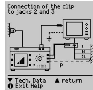
P: potential lead for 4-wire measurement
