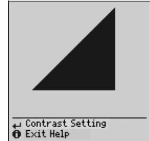
Store the contrast setting to permanent memory with the save function in the setup menu.
