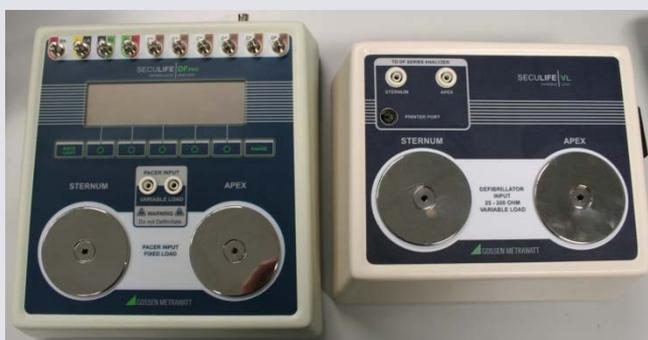
2. Connect the two apex sockets (on SECULIFE VL labeled with "TO DF SERIES ANALYZETR") with the SECULIFE VL cables
