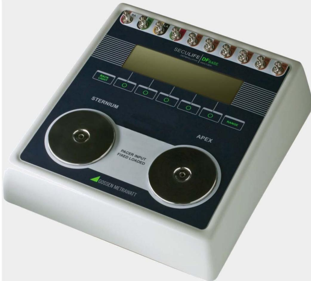
SECULIFE DF<sub>BASE</sub> is a microprocessor-based instrument that is used in the testing of defibrillators. It measures the energy output and provides information about the defibrillator pulse.
