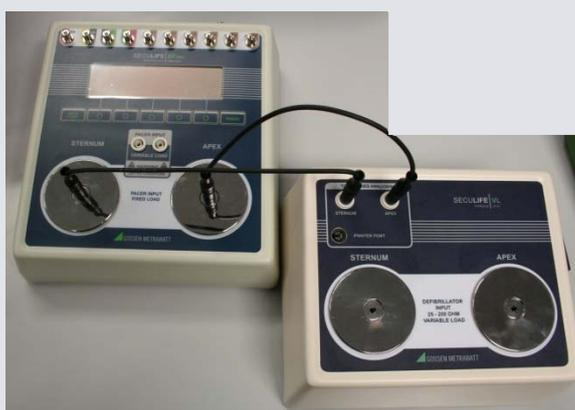
4. Connect the SECULIFE VL –Interface-Cable to the Printer port
