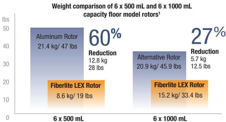
Figure 4: Lower weight advantage of Fiberlite LEX rotors.
