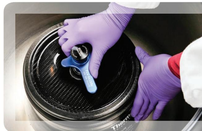
**Figure 9:** Speed handle on rotor lids: Makes tightening the lid safer while also simplifying lid removal.
