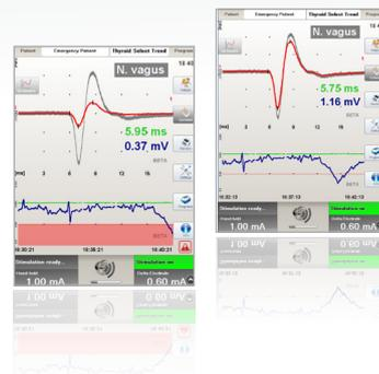
Continuous recurrent laryngeal nerve monitoring made simple. Trend and alarm functions help to detect nerve irritations and early signs of possible nerve impairment. The new nerve detection sound technology provides intuitive feedback for hand-guided stimulation and vagus monitoring. Vagus nerve monitoring may be performed during bipolar electro-cautery without artifact sounds.
