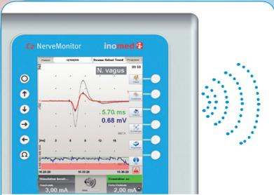
>> **New sound technology** provides intuitive feedback during nerve detection and permits early detection of nerve irritation
